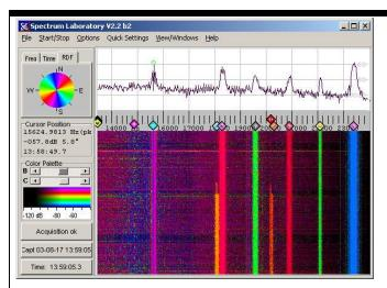
(SpecLab screenshot in "Colour Direction Finder" mode, VLF spectrum, colour~bearing) http://www.gsl.net/dl4yhf/spectra1.html
