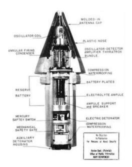
A cutaway view of a Variable Time Fuze.
