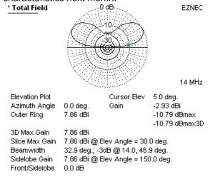
Fig.1. Horizontal Dipole at ½ wavelengths
