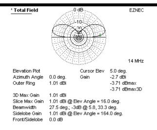
Fig 2.Vertical Dipole at ¼ wavelengths
