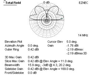
Fig. 3. Vertical Dipole at ½ wavelengths
