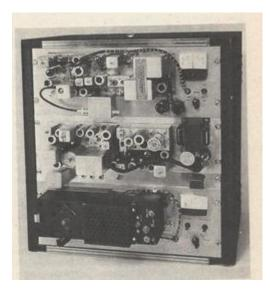
A typical 2 meter repeater in the 1970s often employed surplus commercial repeater equipment. This one uses GE Prog Line transmitter and receiver decks. Those curious metal cylinders are vacuum tube shields. [*The Radio Amateur's Handbook*, 55th ed, 1978]
