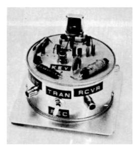
A May 1976 *QST* <u>article</u> by Doug DeMaw, W1CER, described how to build the Tuna-Tin 2 QRP transmitter for 40 meters.
