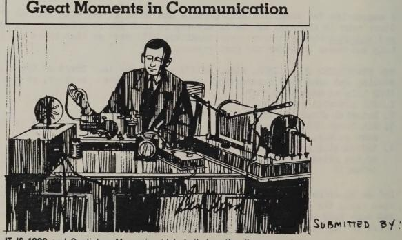
**IT IS 1898** and Guglielmo Marconi, widely hailed as the discoverer of the "wireless," checks out his own receiving apparatus. The heart of his receiver is a device called a "*coherer*," a glass tube of small diameter which contained a small quantity of loosely-packed metallic filings, placed between two metallic electrodes. This coherer detects wireless signals.
